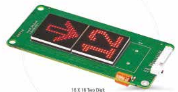
16 X 16 Two Digit Dot Matrix Display
